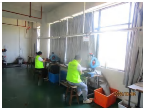
Work process 6 – hole punching
